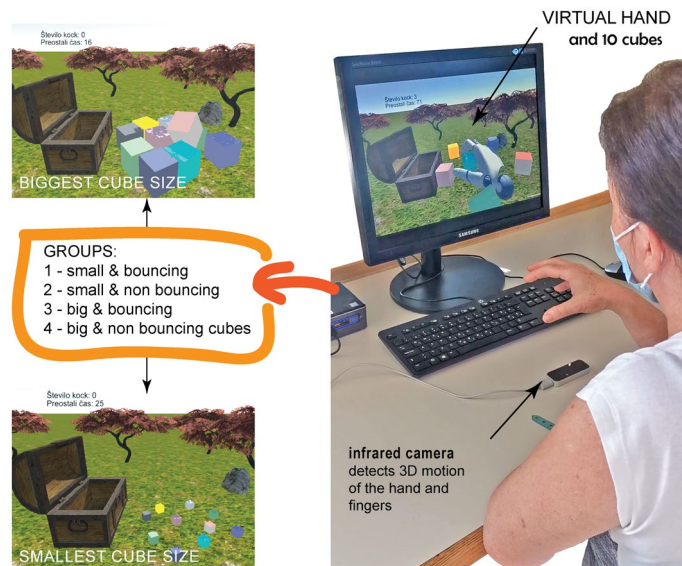
Figure 1. Exergaming setup. LMC detects hand and finger movements for interaction with the virtual environment. Small and large cubes with different bouncing characteristics were used to define 4 variants of the exergame.
