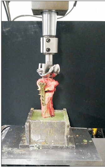
Fig. 2. Testing model mounted on MTS (MTS 858 Bionix; MTS System Co.). A prosthesis for total knee replacement was used for the axial load. The specimen was embedded in polyurethane casting resin and mounted in a fixture.
