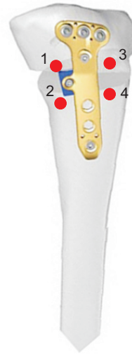
Fig. 3. Schematic drawing of four markers for the displacement measurement (ventral and dorsal sides of both proximal and distal tibial surfaces). 1 and 2 are for posteromedial gap and 3 and 4 are for anterolateral gap.
