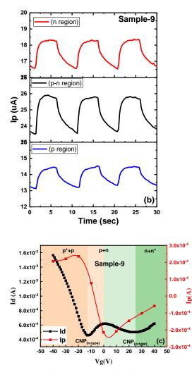
**Figure 8.** Photo-current ( $I_p$ ): (a)  $V_g$  dependent Ip measured for fabricated pn-junction devices (sample-9 and sample-10). (b)  $I_p$  as a function of time with a bias voltage Vd of 1V in the dark and illuminated states during the measurement. The  $I_p$  for the pn-region is readily enhanced because of photo-generated electron-hole pairs in the channel. (c)  $V_g$  dependent  $I_d$  and  $I_p$  for the fabricated pn-junction device (sample-9), for different regions of the device.
