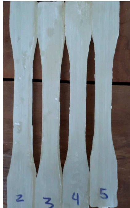
Figure 4. Specimens nanocomposites with 1 wt% of CNCs for tensile test.
