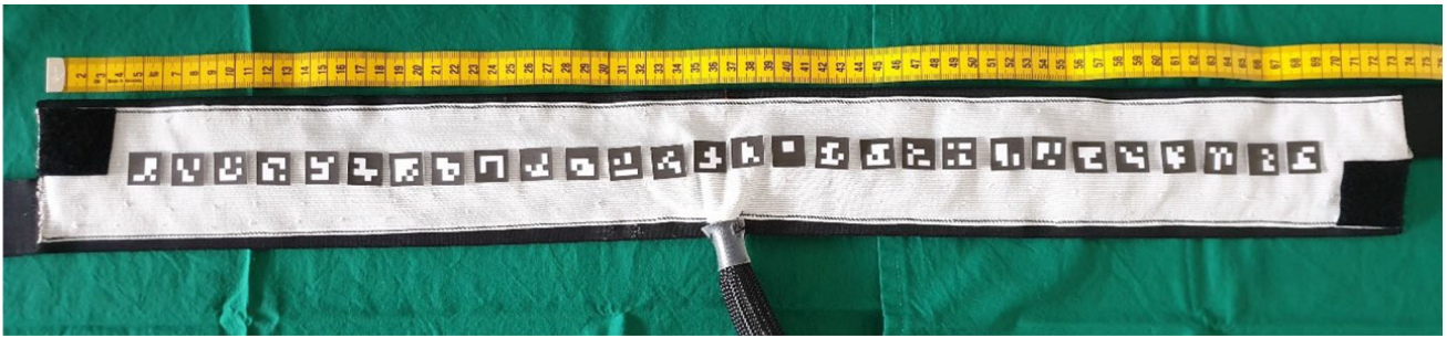
Fig. 1 EIT belt with ArUco markers on electrodes and measuring tape
