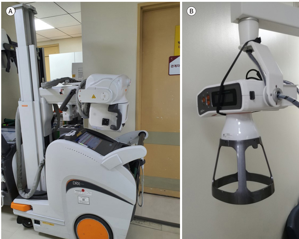
Fig. 1. Images of a traditional mobile digital X-ray device (A) and a camera-type portable X-ray device (B).
