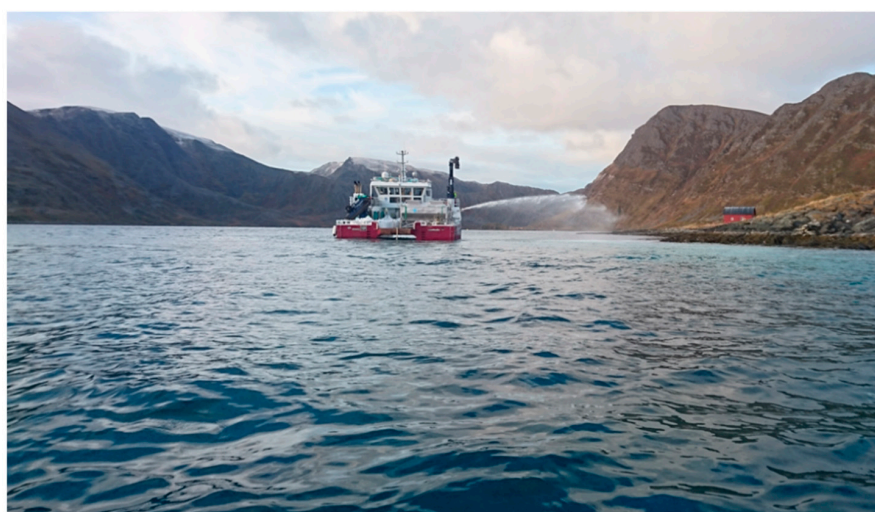
Figure 18. Photo of the boat spraying lime suspension of coarse \text{CaO} over the sea.
