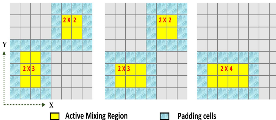
Fig. 3 Synthesis steps for typical bio-operations on DMFB
