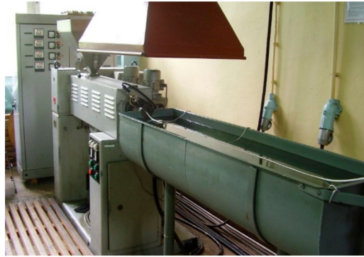
Figure 2. Station for testing the process of microcellular extrusion.
