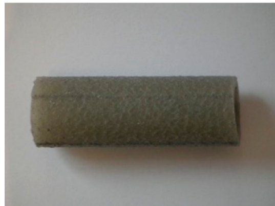
Figure 6. A fragment of the outer layer of a porous pipe with visible metal grains.
