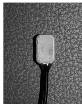
FIGURE 1 Cartilage conduction hearing aid and its transducer. A. The cartilage conduction hearing aid and its appearance when used by the patient (right). B. A plain transducer that was used for the current measurements. The same model of the transducers is used for cartilage conduction hearing aids
