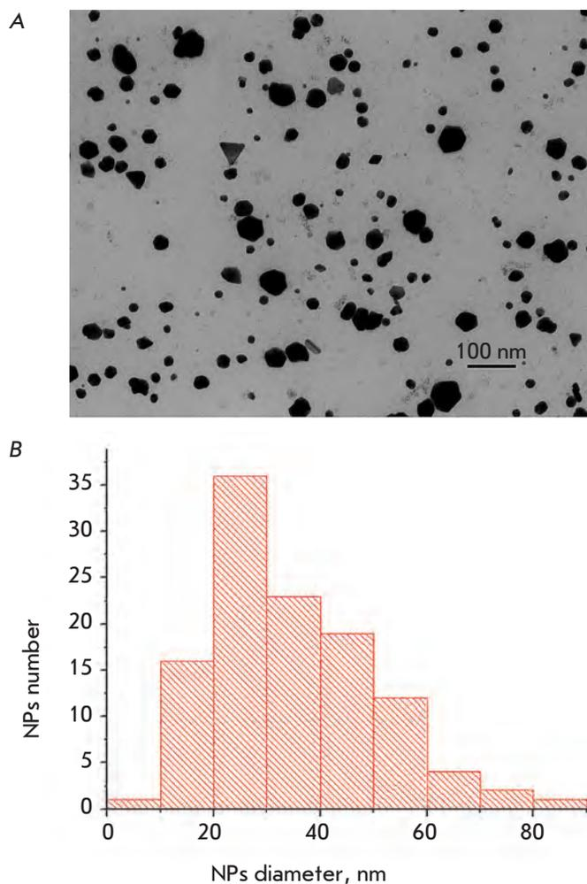
**Fig. 1.** Transmission electronic microscopy of silver NPs preparation Argovit®. NPs image (A) and diameter distribution (B). Electron microscope JEM-100CX ("Jeol", Japan), accelerating voltage 80 kV. Data obtained by prov., D.Sc. Dzantiev B.B., RAS Institute of biochemistry, Moscow
