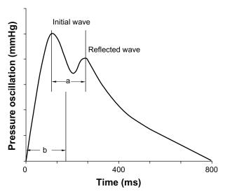
**Figure 1** Methods of measuring the oscillometrically generated pulse wave. **Notes:** a = difference in the time between the pressure peak of the first wave and the reflected wave; b = difference in the time between the beginnings of each wave.
