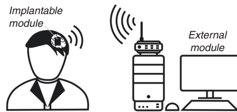
Fig. 1 Illustration of a brain-implantable system, including an implantable module and an external module communicating with each other through wireless connection. In general, the implantable module is configured by the external module through wireless connection. It may also wirelessly receive electric power from the outside. The implantable module comprises a microelectrode array for extracellular recording of neuronal activities, and the electronic circuitry supporting its function. The electronic part usually includes a neural signal preconditioning block, which pre-amplifies the signals sensed by the electrode array, filters out the out-of-band frequency components, and finally digitizes the signals using per-channel or time-shared analog-to-digital converters. After digitization and some signal processing tasks, the recorded signals are telemetered through a wireless link to the external module.
