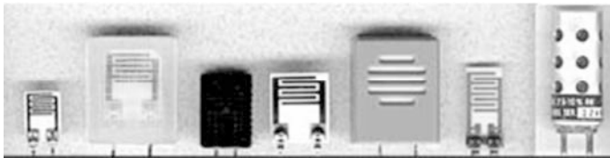
Fig. 4.38. Resistive sensors are based on an interdigitated or bifilar winding. After deposition of a hygroscopic polymer coating, their resistance changes inversely with humidity. The Dunmore sensor (far right) is shown 1/3 size (reprinted from (Roveti, 2001), Copyright 2001, with permission from Questex Media Group, Inc.)
