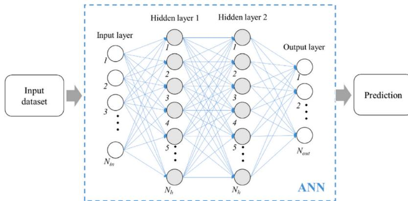
Fig. 8. Typical architecture of the multilayer perceptron (MLP) model.
