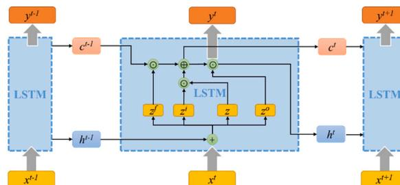
Fig. 3. Illustration of LSTM architecture;  $x^t$ ,  $y^t$ ,  $c^t$ , and  $h^t$  represent the input, output, cell state, and hidden state at time step  $t$ , respectively.
