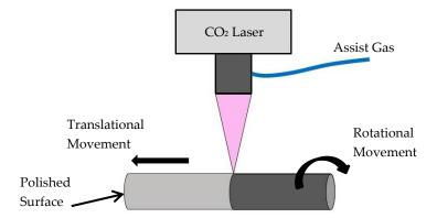
**Figure 1.** Schematic diagram for the CO<sub>2</sub> laser polishing scan process of additive manufacturing (AM) produced stainless steel 316L cylindrical samples.
