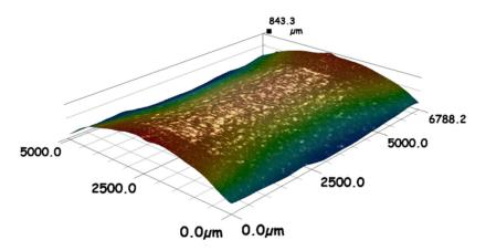
**Figure 4.** Three-dimensional (3D) microscope image of 316L SST AM sample after CO<sub>2</sub> laser polishing with 110 W, 20% percentage overlapping laser scans (OV), 20 rpm, and laser beam focused on the surface.
