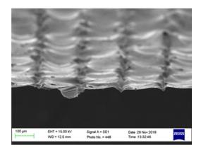
Figure 9. SEM image of a remaining unmelted particle due to lack of fusion.
