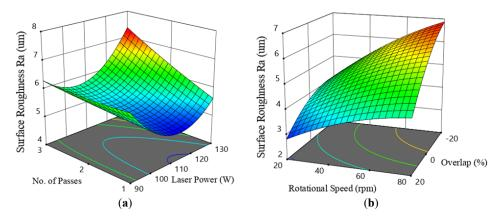
**Figure 11.** Response surface model (RSM) graphs (**a**) related to design of experiment (DoE)-1 in Table 2, showing the interaction effect on Ra of the laser beam power and the number of passes at 50 rpm; and (**b**) related to DoE-2, the effects of rotational scanning speed and the percentage overlap, with the focal position set on the sample surface.
