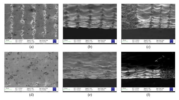
**Figure 7.** SEM micrograph showing the top and side views of AM 316L SST samples polished with 50 rpm, 0% overlap, one scanning pass, and 90 W in (**a**) top, (**b**), and (**c**) side-view, as well as 130 W in (**d**) top, (**e**), and (**f**) side view.
