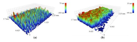
**Figure 13.** Three-dimensional (3D) optical images of the surface topography of (**a**) as-built and (**b**) laser polished samples.
