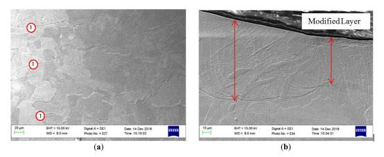
**Figure 10.** SEM micrograph of the cross-section of the (**a**) as-received and (**b**) re-melted modified layer of the polished sample processed with 110 W, 20 rpm, 20% OV, and the laser beam focal positioned on the sample surface.
