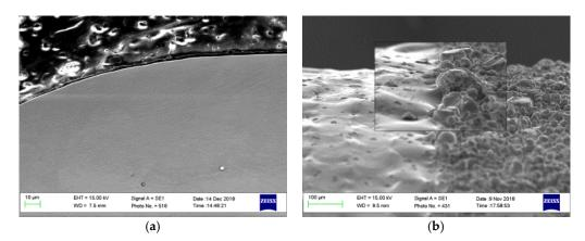
**Figure 8.** SEM micrograph shows (**a**) the cross-sectional view of the polished sample and (**b**) the side view. This sample was processed with 110 W, 20% overlap, and 20 rpm, and the laser beam was focused on the sample surface.
