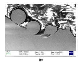
**Figure 5.** (a) Scanning electron microscopy (SEM) micro-image of the metal AM sample surface showing (a) the surface morphology with the fully melted material in the back ground, zones (1) and (2) show the BALLING effect and the partially melted and adhered neighboring particles, (b) shows the cross-section SEM micrograph view of the same surface, zone (3) shows unmelted powder particles, and (c) shows a high magnification from the micrograph shown in (b).
