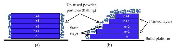
Figure 14. (a) Printing in the vertical direction and (b) printing curvature geometry.
