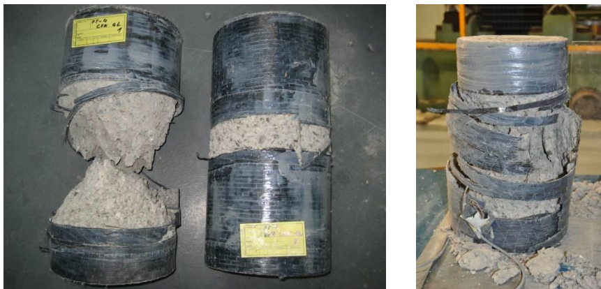
Figure 10. Typical failure of CFRP-confined plain concrete cylinders.
