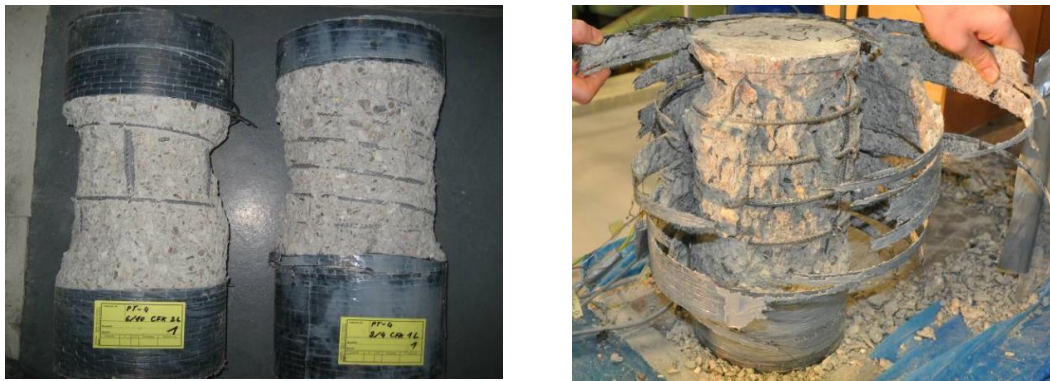
Figure 11. Typical failure of CFRP-confined RC cylinders.
