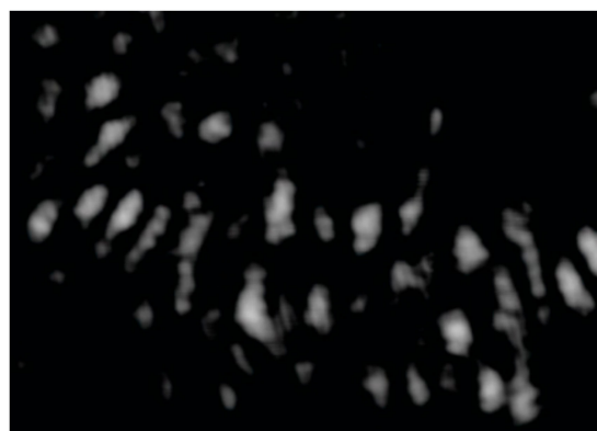
Figure 3. Interferogram partially captured by a CMOS camera at the output end of the capillary, while the inner air pressure of the capillary elevates from 400 to 1012 hPa. Video S1 in the Supplementary Materials.
