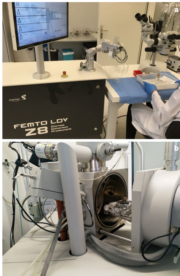
Figure 1. (a) Standardised lab set up for ex-vivo porcine eye surgeries. (Permission obtained from Ziemer AG, Switzerland for displaying the brand logo). (b) Porcine cornea mounting on the Scanning Electron Microscopy.
