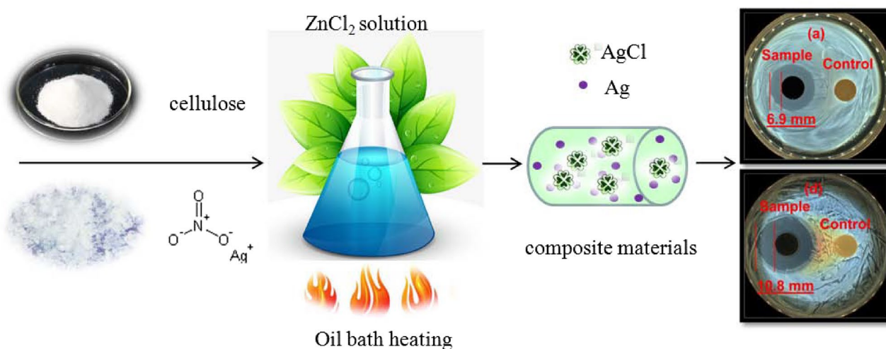
Figure 4. The schematic illustration of the formation process of Ag@AgCl-reinforced cellulose composites in the present strategy. (The illustration is drawn by ourselves).
