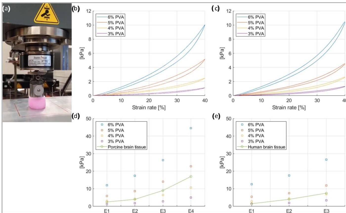
**Figure 4.** (a) PVA sample under test. (b) Strain-rate curves of the mechanical tests on the PVA samples at 0.01/s. (c) Strain-rate curves of the mechanical tests on PVA samples at 0.083/s. (d) Elastic moduli ( $E_i$ ) of PVA samples at 0.01/s, compared to porcine brain tissue properties found in the literature. (e) Elastic moduli ( $E_i$ ) of PVA samples at 0.083/s, compared to human brain tissue properties found in the literature.
