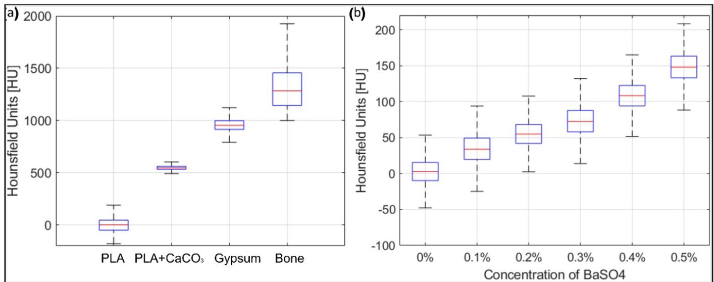
**Figure 6.** (a) Boxplots related to the X-ray attenuation, in Hounsfield units, of the materials for building the skull phantom. (b) Boxplots related to the X-ray attenuation, in Hounsfield units, of the mixtures for producing the brain.
