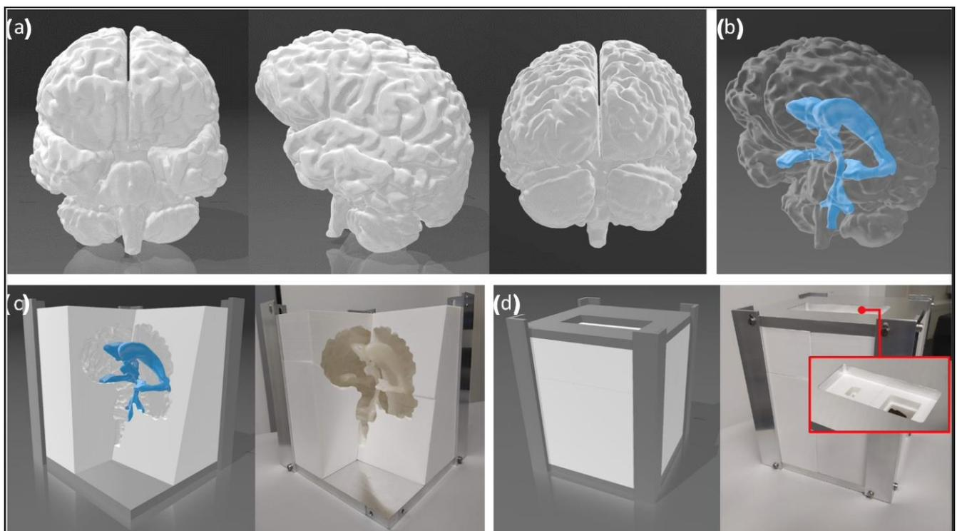
**Figure 3.** (a) Computational model of the brain, segmented from the MR image. (b) Computational model of the ventricles, located inside the brain. (c) Inside view of the computational model of the brain mold and corresponding inside view of the 3D-printed brain mold. (d) Outside view of the computational model of the brain mold and corresponding outside of the 3D-printed brain mold. The red frame shows the large and small openings at the top.
