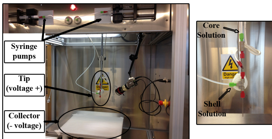
Figure 5. Electrospinning experimental set-up with its main components: syringe pumps, tip and collector. Coaxial injection capillaries can be used (image on the right) to fabricate nanofibrous core-shell structures.
