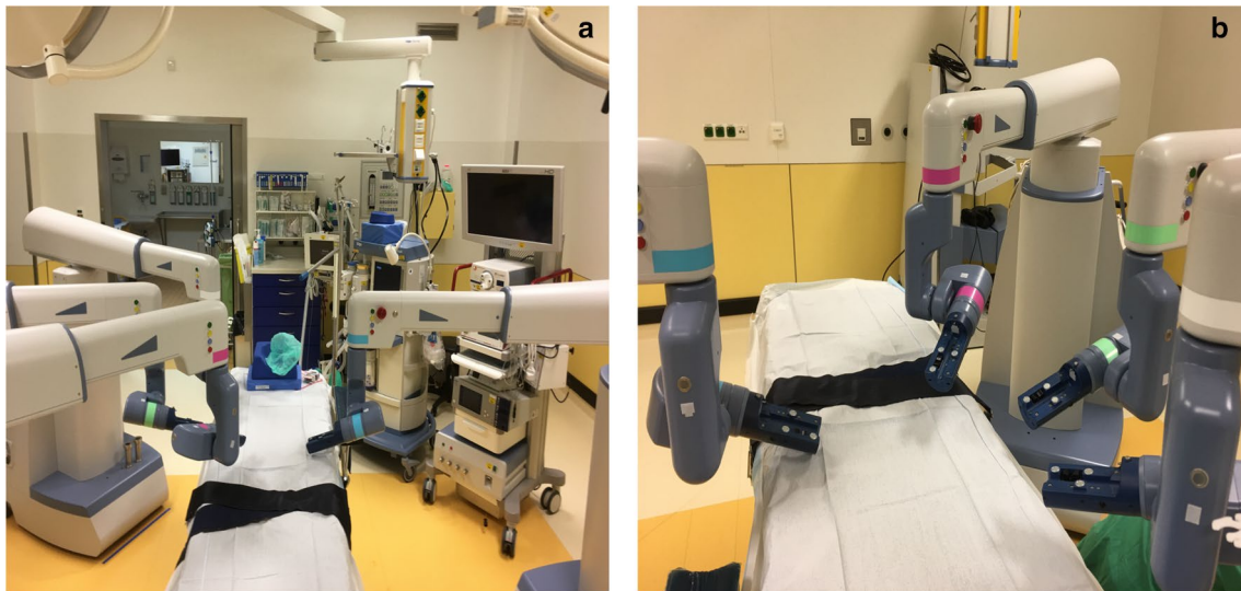
Fig. 4 A view of the designated positions of the robot arms. a The arc formed array of three arms on the table's right side with the laparoscopy tower shown on the upper left side and the fourth arm on the table's left side; b a closer view of the arms with the console in the background
