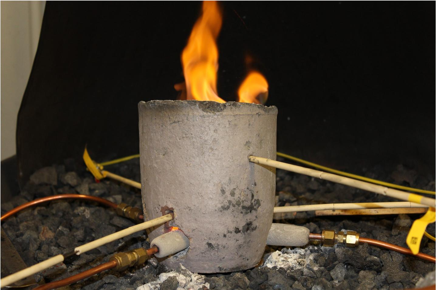
**Fig 4. Experimental tuyères and furnace.** Experimental tuyère and furnace setup, at the MIT metallurgy forge in the Department of Materials Science and Engineering. Photograph by Elizabeth Paris.
