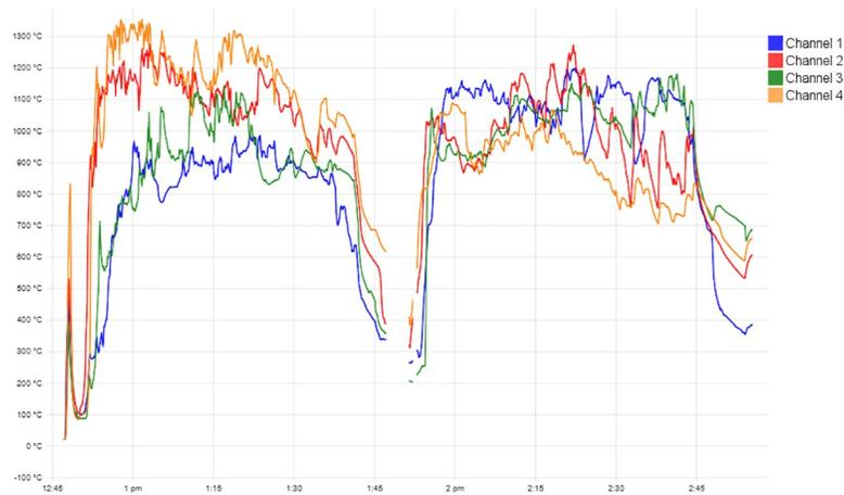
**Fig 11. Temperatures reached using experimental tuyères.** Results of the replication experiments with experimental tuyères, showing sustained temperatures above the melting point of copper. Temperatures from the thermocouples were recorded using PicoLog 6 software.
