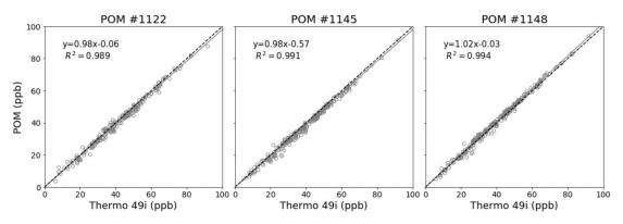
Figure 6. Post-deployment co-location correlation plots for 1-h O<sub>3</sub> concentrations.
