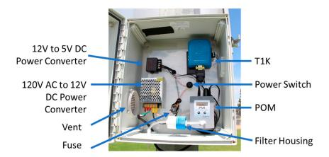
Figure 1. Ozone sensor node with labeled components.
