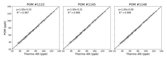
**Figure 4.** Pre-deployment co-location correlation plots for 1-h O<sub>3</sub> concentrations after the in-situ field calibration was performed.
