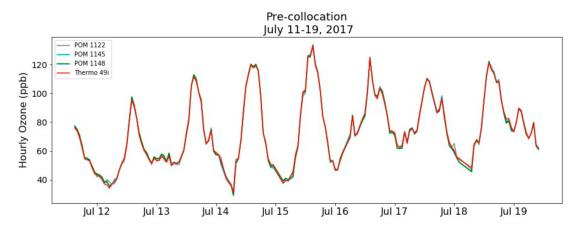
**Figure 3.** Pre-deployment co-location at Crestline time series for 1-h mean O<sub>3</sub> concentrations after the in-situ field calibration was performed.
