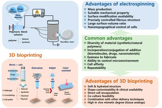
**Figure 1.** Relative comparison of technical advantages between electrospinning and 3D bioprinting to engineer skeletal muscle tissue constructs.
