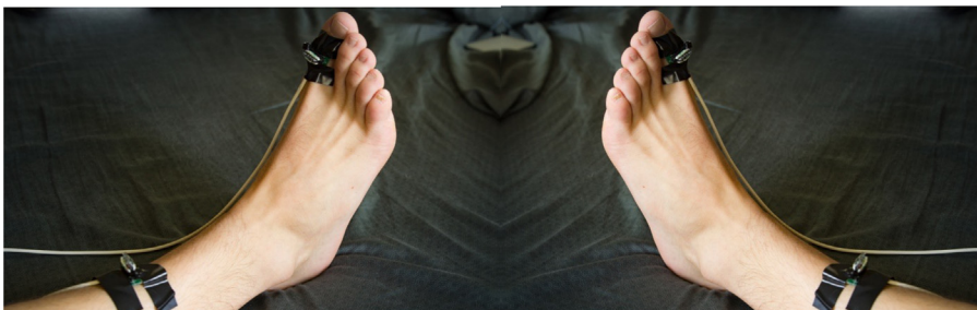
Fig. 17. (Left panel) Placement of accelerometer evaluation boards on the anterior surface of the right tibia two inches proximal to the medial malleolus and on the dorsal surface of the proximal phalanx of the right big toe. (Right panel) Placement of accelerometer evaluation boards on the anterior surface of the left tibia two inches proximal to the medial malleolus and on the dorsal surface of the proximal phalanx of the left big toe.
