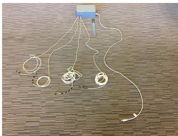
Fig. 3. Metal box housing covering low-cost, portable, USB/ethernet data logger system [26] (Fig. 5) with four 16-foot-4.5-inch light, shielded cables identified with one, two, three, or four bands of black tape to connect input from accelerometer evaluation boards board [25] (Fig. 1) on left and a standard 6' hi-speed USB revision 2.0 shielded 28AWG/ 2C+24AWG/2C (UL) E305668 type CM 75 °C CSA 204790 type CM 75 °C MSL cable to connect output to a laptop computer on right. A one-foot ruler is displayed by the equipment.
