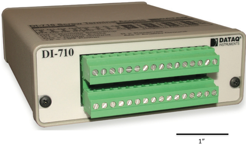
Fig. 4. A low-cost, portable, USB/ethernet data logger system (Fig. 5) [26] for accelerometry data acquisition.
