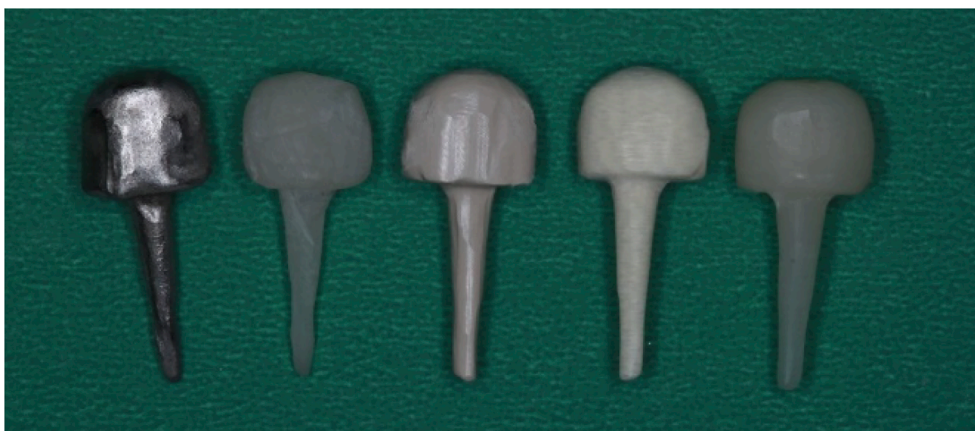
Fig. 2. CAD/CAM fabricated posts utilized in this study. From left to right Cast Metal post-core, Vita Enamic post-core, PEKK post-core, Trilior post-core, Shofu HC post-core.
