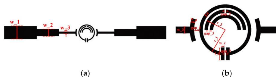
**Figure 1.** Structure of the proposed microwave sensor. (a) The full view of the microwave sensor; (b) the SRR structure and the sensing zone of the sensor.
