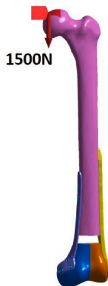
Fig. 4. The axial loading of 1500 N at the femoral head [20].
