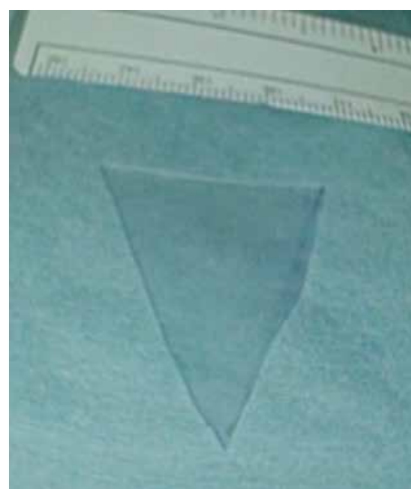
FIGURE 3: The silicone plate (200×150 mm silicone sheet with a thickness of 0.5 mm; Koken Co., Ltd. Bunkyo ward, Tokyo, Japan) was molded into an inverted triangle, comparable to the shape of the uterine cavity.
