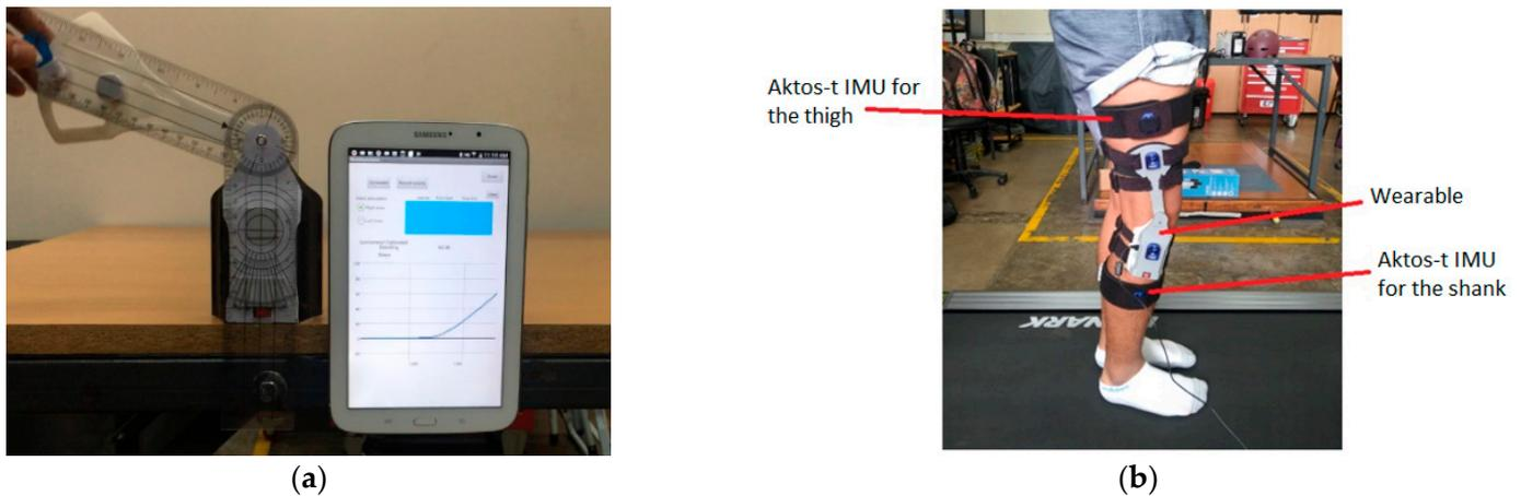
**Figure 6.** (a) Set up for the comparison of the wearable and the commercial goniometer; (b) set up for testing of the AROM. The wearable and the Aktos-t are worn by the subject.
