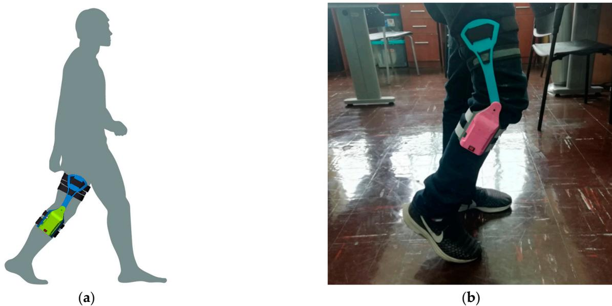
Figure 2. (a) 3D model of a person using the wearable; (b) a user wearing the wearable goniometer.
