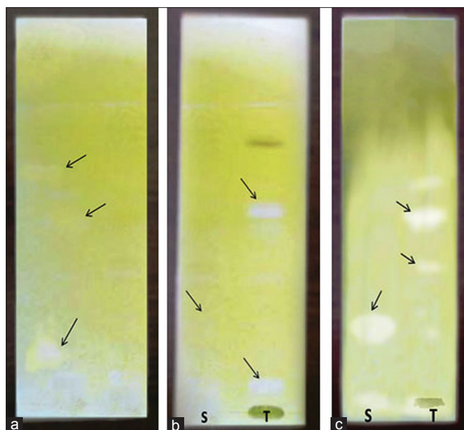
Figure 3: Thin layer chromatography bio-autography plate showing (a) false inhibition activity (b) acetylcholinesterase inhibition activity (c) butyrylcholinesterase inhibition activity; S = Standard galantamine solution, T = Test solution of methanol extract, (→) indicates white spot on TLC plate which corresponds the positive (plate b and c) or negative (plate a) result of the chemical reaction
