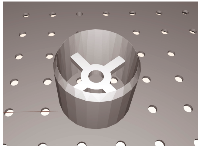
Figure 2. The STL file format of the digital models of the cookie cutters. STL, standard tessellation language.
