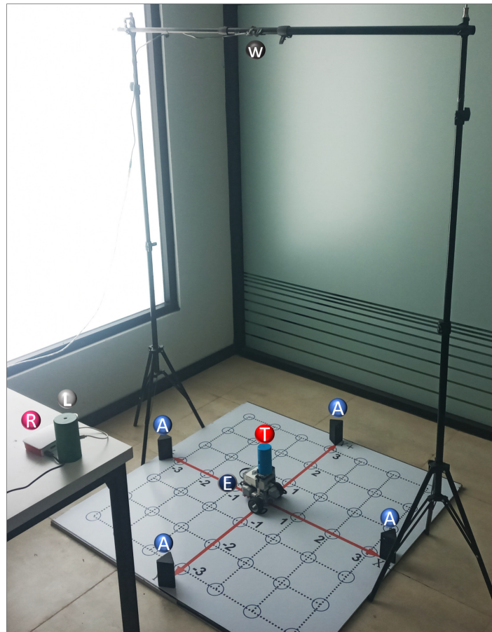
Figure 5. Hardware setup: anchor devices (A), tag device (T), EV3IA (E), listener device (L), Raspberry Pi (R), and webcam (W).
