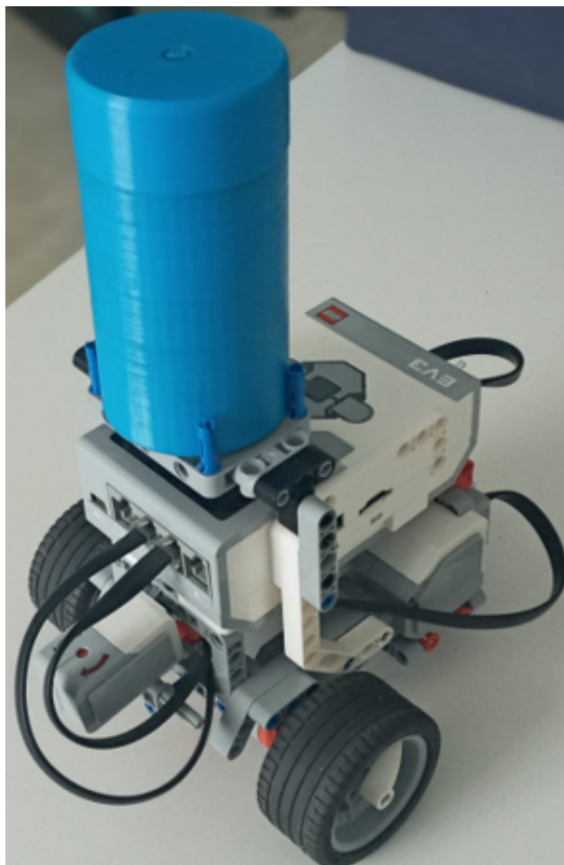
Figure 12. EV3 interactive actuator model equipped with a tag device and a gyroscope sensor.
