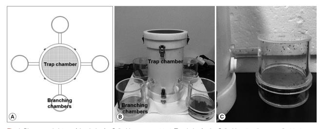
Fig. 1. Diagram and picture of the device for *Culicoides* movement test. The device for the *Culicoides* attraction or repellent tests consisted of a main trap chamber and 4 branching chambers (A, B). *Culicoides* were collected in the trap chamber and allowed to move to the branching chambers containing each test substance (C).
