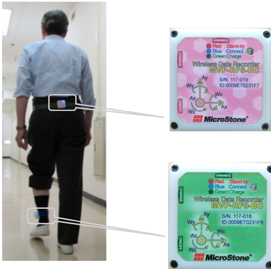
FIGURE 1 Attachment positions of the triaxial sensors
