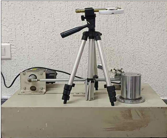
Figure 3: Setup of custom fabricated cyclic fatigue device
