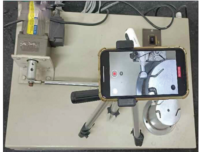
Figure 4: Video recorder for calculation of the time to fracture ( T )
