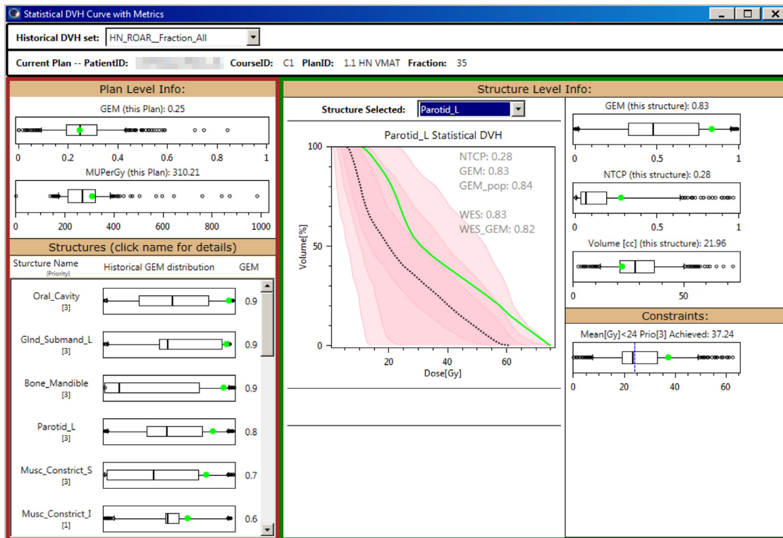
Figure 1 Statistical dose-volume histogram (DVH) dashboard quantifies comparison of statistical metrics for the current plan (green) versus historical experience. Statistical DVH (center) compares the DVH curve to historical experience for the median (dashed line), 50% confidence interval (CI; dark pink), 70% CI (intermediate pink), and 90% CI light pink. Box-and-whisker plots compare plan level (left panel) and structure level (right panel) metrics.
