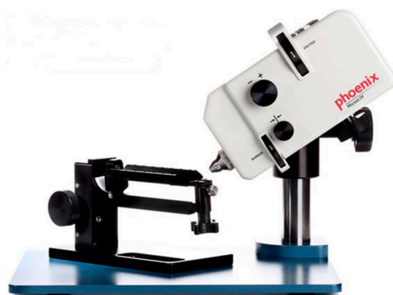
Figure 3. Physical photos of a Micron II rodent retinal imaging microscope.
