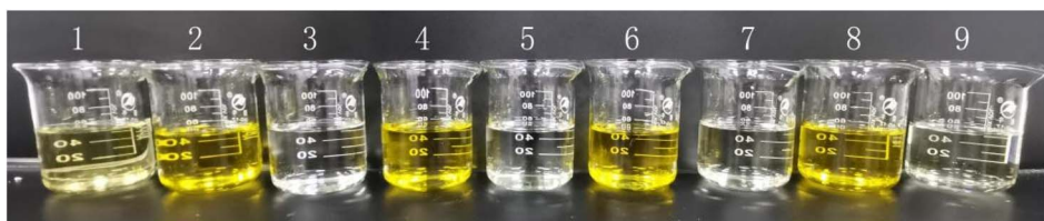
Fig. 9 Decolorization effect of 200D, 400D, 600D, and 800D NFs on the raw synthetic solution. Number 1 is the raw synthetic solution, numbers 2, 4, 6, and 8 are the concentrated solutions of 200D, 400D, 600D, and 800DNFs, numbers 3, 5, 7, and 9 are the permeate solutions of 200D, 400D, 600D, and 800D NFs
