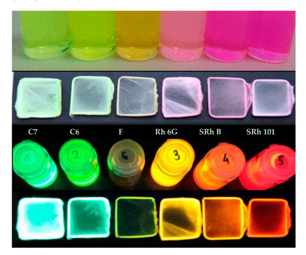
**Figure 2.** Images of the polymer solutions and the corresponding electrospun submicronic fiber mats collected on copper frames in visible light (**upper**) and UV light (**lower**).
