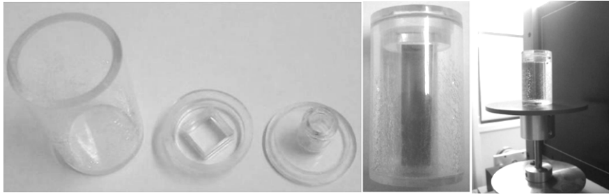
Fig. 1. Cylindrical phantom (left) with FXG vial (middle) for \mu CT setup (right).
