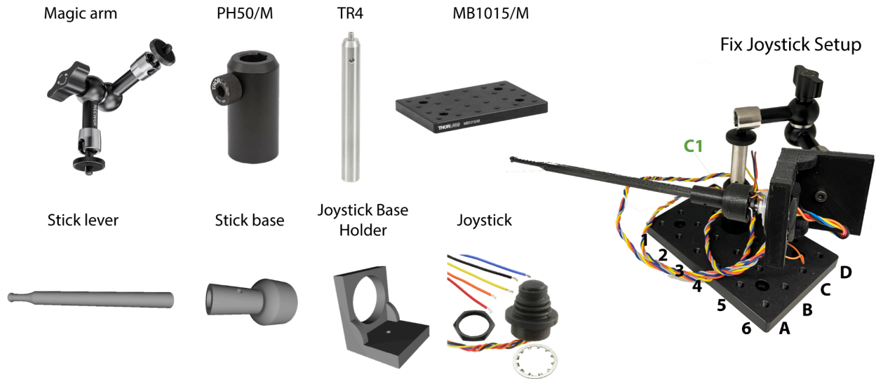
Figure 2. Fixed Joystick setup assembly
