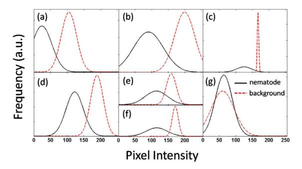
**Figure 2. Pixel intensity distributions of nematode and background environment.** Plots (**a**) through (**g**) correspond to distributions obtained from the images of Fig. 1. Grayscale pixel intensities vary between 0 (black) and 255 (white). Distributions are assumed to be Gaussian and parametrized with the mean and standard deviation of pixel intensities. doi:10.1371/journal.pone.0011631.g002
