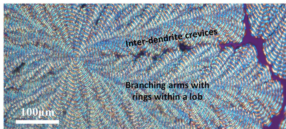
**Figure 3.** POM graph showing multiple-lobe dendritic banded PPDO growing lengthwise (crystallized from PPDO/PVPh = 80/20,  $T_c = 80\text{ }^\circ\text{C}$ ).
