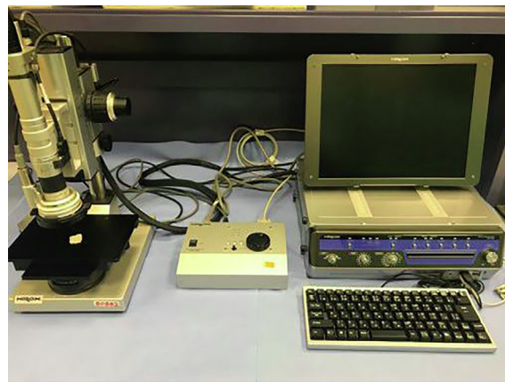
Fig. 3 Hirox digital microscope for assessment of casts.
