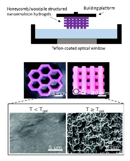
**Figure 4.** SLA 3D printing of honeycomb and woodpile structured hydrogels using thermoresponsive nanoemulsion inks (modified from [59]).
