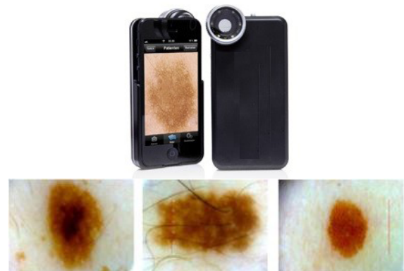
FIGURE 2. The dermoscope device attached to the iPhone and sample of images captured using the device.
