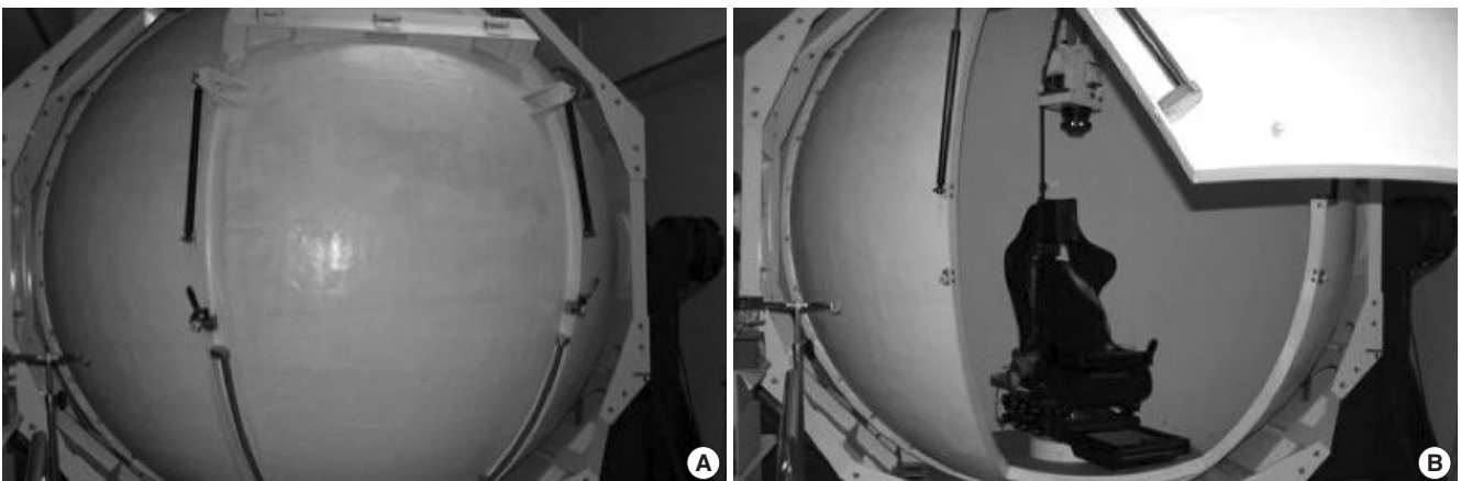
Fig. 7. The hydraulic driven spherical dome for examining the off vertical axis rotation (OVAR). The seen of outside (A) and the inside (B) of the dome.
